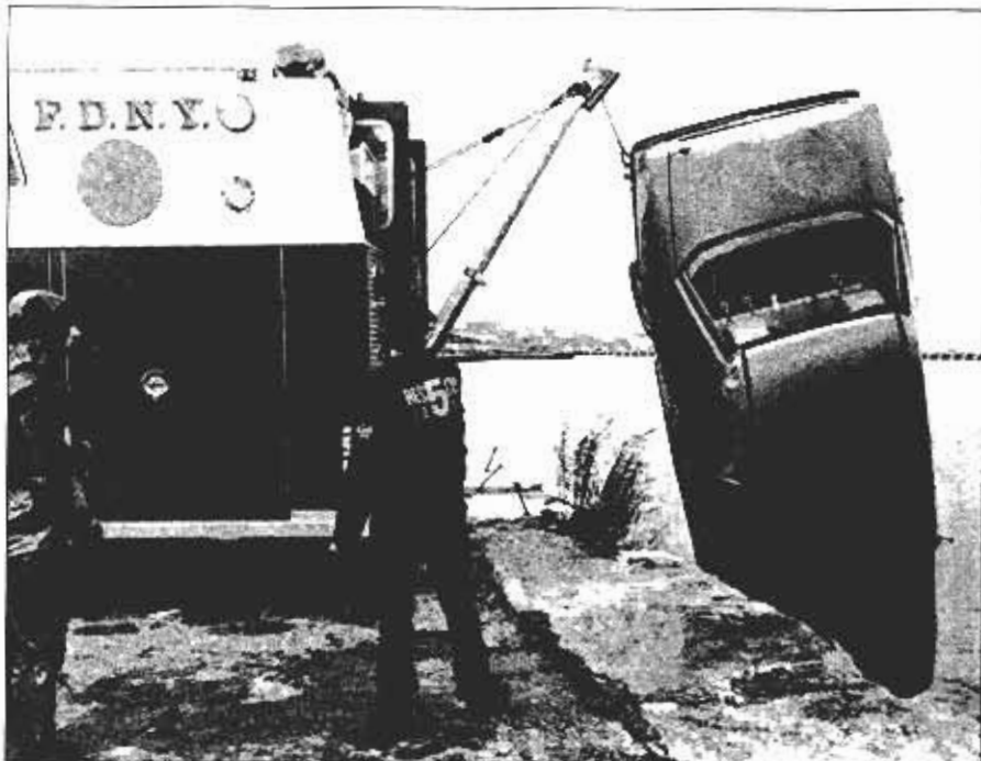
Your own apparatus can serve as a crane when equipped with proper fittings to support an A-frame assembly from which any type of pulley system can be adopted. (Photo by John Skelson.)
