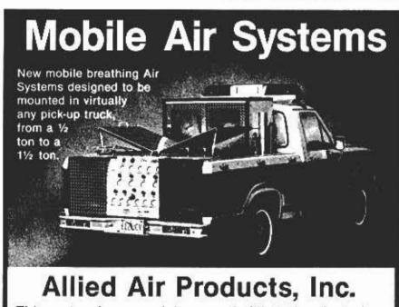
This system is a complete cascade fill station, featuring 7 to 22 SCFM compressors, SCBA storage, storage system. 3600-5000 PSI, with the capability of filling 4 SCBA bottles at one time. For more information call or write us today.
